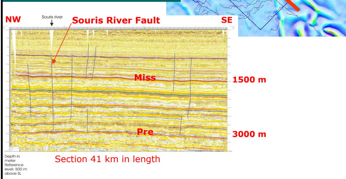
**Figure 1.** Correlation of fault on a depth migrated seismic (Line SOU-06) with magnetic and lineament correlation (N/S segment of the Souris River), in the Assessment Area. Basement is at a depth of about 3000 m subsurface and the Mississippian is at roughly 1200-1500 m depth subsurface. Elevations in the area are 600-800 m.
