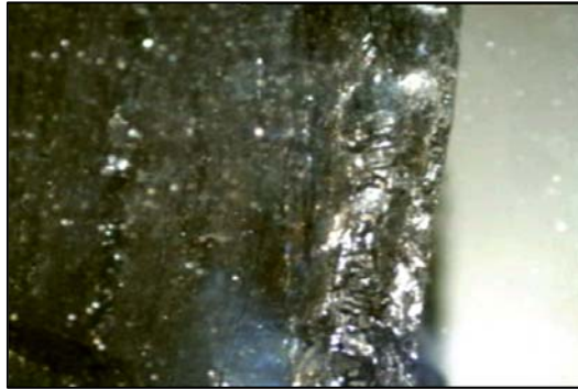
Figure 8. Representative photomicrograph of a sub-bituminous coal that is undersaturated (i.e. held in region A in Figure 8). Image is 7.2 mm wide.
