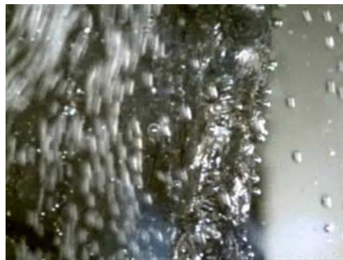
Figure 9. Representative photomicrograph of a sub-bituminous coal that is producing gas (i.e. held in region B in Figure 8). Image is 7.2 mm wide.
