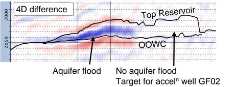
Figure 1. Direct evidence for an acceleration infill target (unswept area) at Gannet F.
