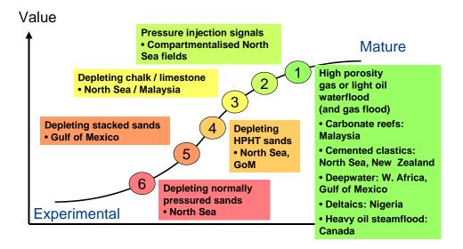
Figure 2. A maturity S-curve for different 4D applications. (For simplicity here, we only show only high porosity waterflood / gasflood. Lower porosity waterflood / gasflood reservoirs (e.g. <22% porosity) would sit further down the curve due to the smaller 4D signal).
