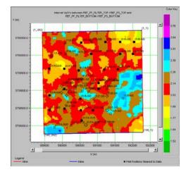
Figure 4.  $V_P/V_S$  between top and bottom horizons from filtered PP and PS data.
