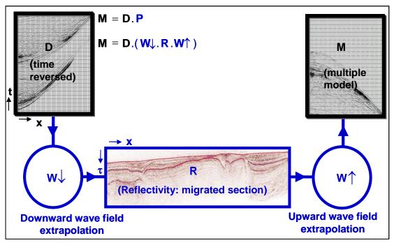
Figure 1. Principles of the model-based surface related multiple prediction using regularized shot records as an areal source for the demigration procedure.
