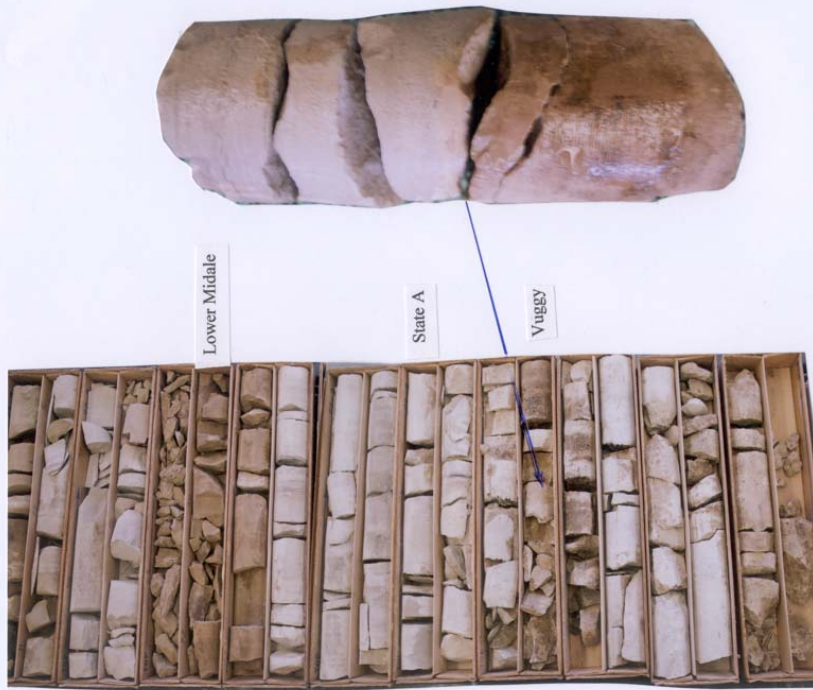
Oil is contained within Lower Midale mudstones. The State A is composed of a thin package of tight stacked argillaceous mudstones. Note erosional contact between tight argillaceous mudstone of the State A and the oil-stained Frobisher Vuggy Porosity. (4662').
