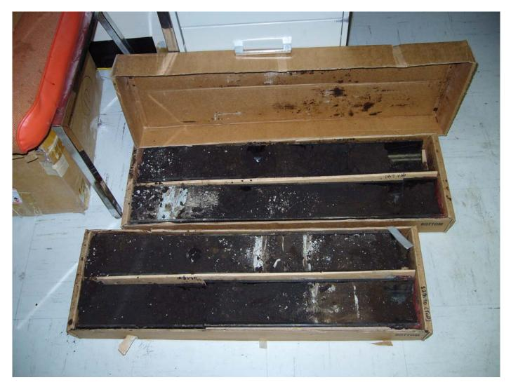
Figure 3. Boxes of core taken from the Bakken formation at Plover Lake Field.
