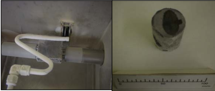
(a) Trimming (b) Oil Sand Plug Figure 3. Oil sands sample plug.
