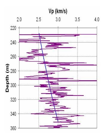
Figure 3. P wave velocity versus depth.
