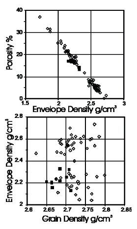
Figure 4. Top Panel: Porosity as a function of envelope density.
