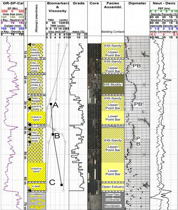
Figure 3. Composite Log 05-1519. Reservoir heterogeneity controls not only the bitumen grade but also quality of the bitumen. Viscosity increases down the hole (points A, B and C) and appears to be the intensified in the best reservoir facies. Biomarker analysis suggests the presence of 3 compartments. From bottom to top the first compartment comprises geochemical samples 2-5, the second 6-8, and the third sample 9. Biodegradation intensifies down the each compartment.
