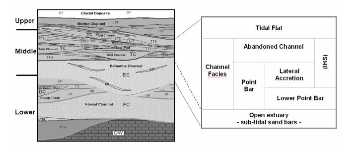
Figure 2. Schematic 2D depositional diagram of McMurray Formation broken into its constitutional units: continental (lower McMurray Formation), estuarine (middle McMurray Formation) and marine (upper McMurray Formation). The right side of diagram shows major architectural elements that comprise the most heterogeneous sediments deposited in estuarine setting. Modified chart courtesy of Albian Sands Energy Inc.
