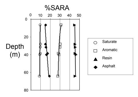
Figure 4. Well 05-1519. latroscan (SARA) bulk composition for bitumen versus depth
