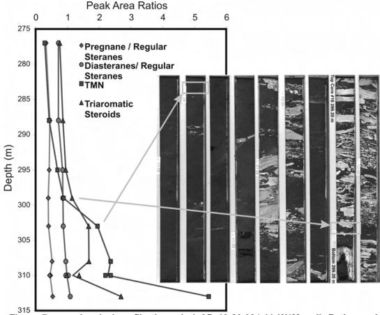
Figure 7. geochemical profile through 1 AD 13-26-084-11 W4M well. Ratios and abundance of certain biomarkers indicates increased biodegradation down the hole.
