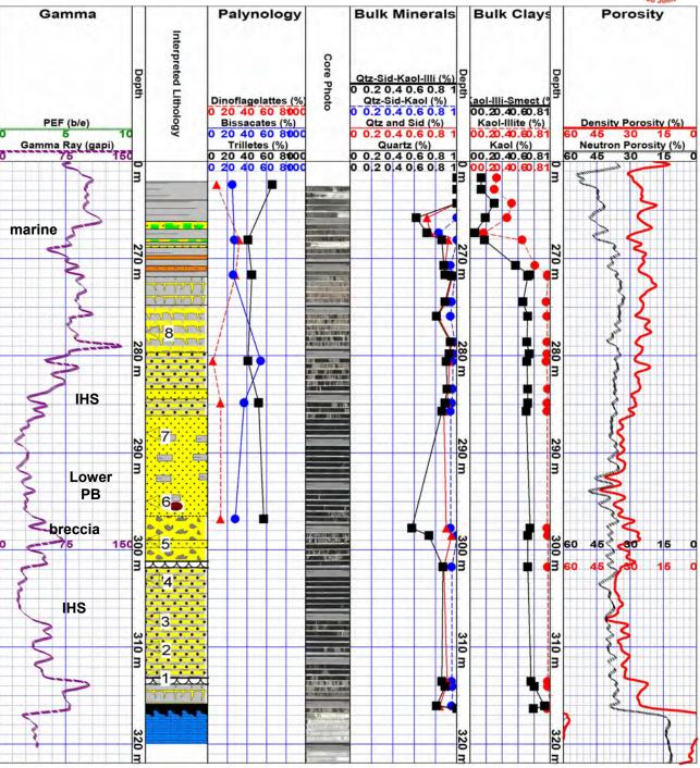
Figure 6. 1 AD 13-26-084-11 W4M. Reservoir heterogeneity inherited from depositional processes is reflected by distinct sedimentary structures and ichnofacies, and confirmed by mineralogical, palynological and petrophysical data. Numbers 1-8 are sample points used to create a geochemical compositional profile presented in Figure 7.
