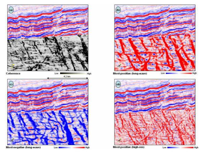
**Figure 3.** Zoom of chair-displays where the vertical display is an inline from the 3D seismic volume and the horizontal displays are time slices through (a) coherence (b) most-positive (long-wavelength) (c) most-negative (long-wavelength) (d) most-positive (shortwavelength) curvature attribute volumes. Note how the fault lineaments correlate with the upthrown and downthrown signatures on the seismic.
