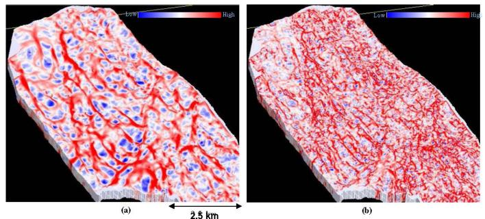
**Figure 1.** Comparison of (a) long-wavelength and (c) high-resolution most-positive curvature strat-cube displays from a 3D volume from Alberta. The finer detail in terms of fault/fracture lineaments could be useful for certain objectives. The upper surface is close to 1550 ms.
