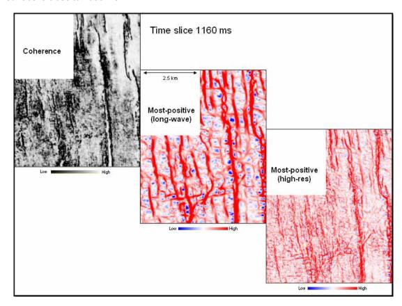
**Figure 2.** Comparison of (a) coherence (b) most-positive curvature (long-wavelength) and (b) most-positive curvature (shortwavelength) horizon slice displays from a 3D volume from Alberta.
