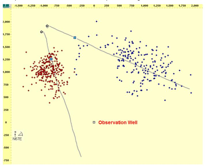
Integration of the microseismic data with other reservoir information including seismic reflection volumes also offers the possibility to understand the impact of reservoir structure on the hydraulic fracture geometry.
