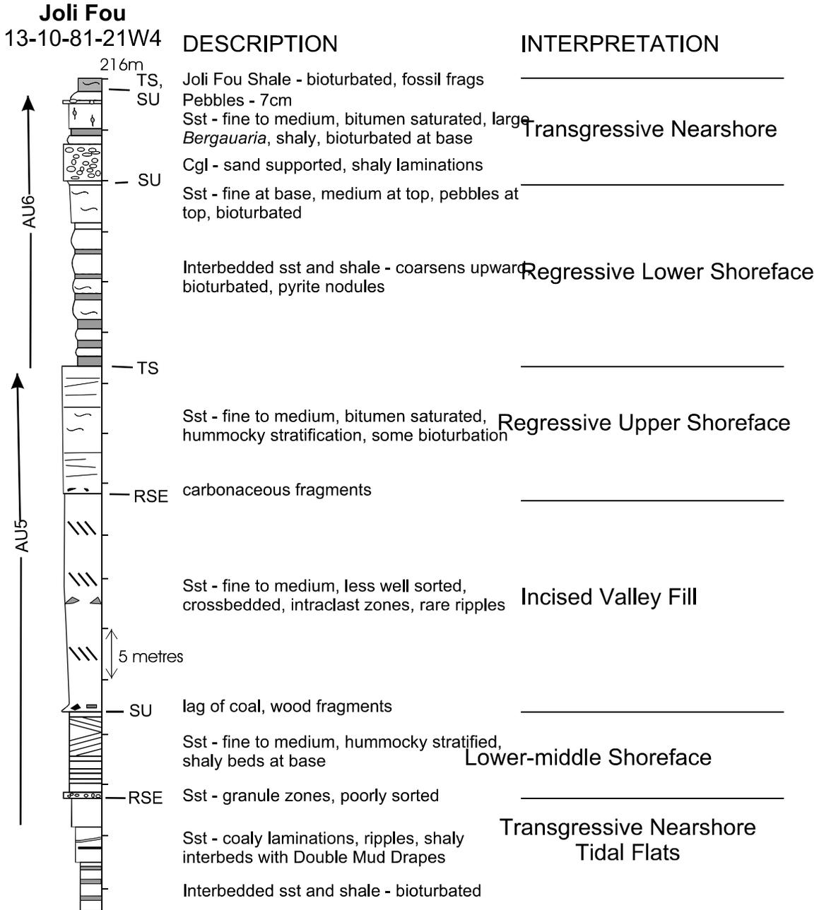
Figure 5: Core log showing amalgamated valley-fill sands and shorefaces
