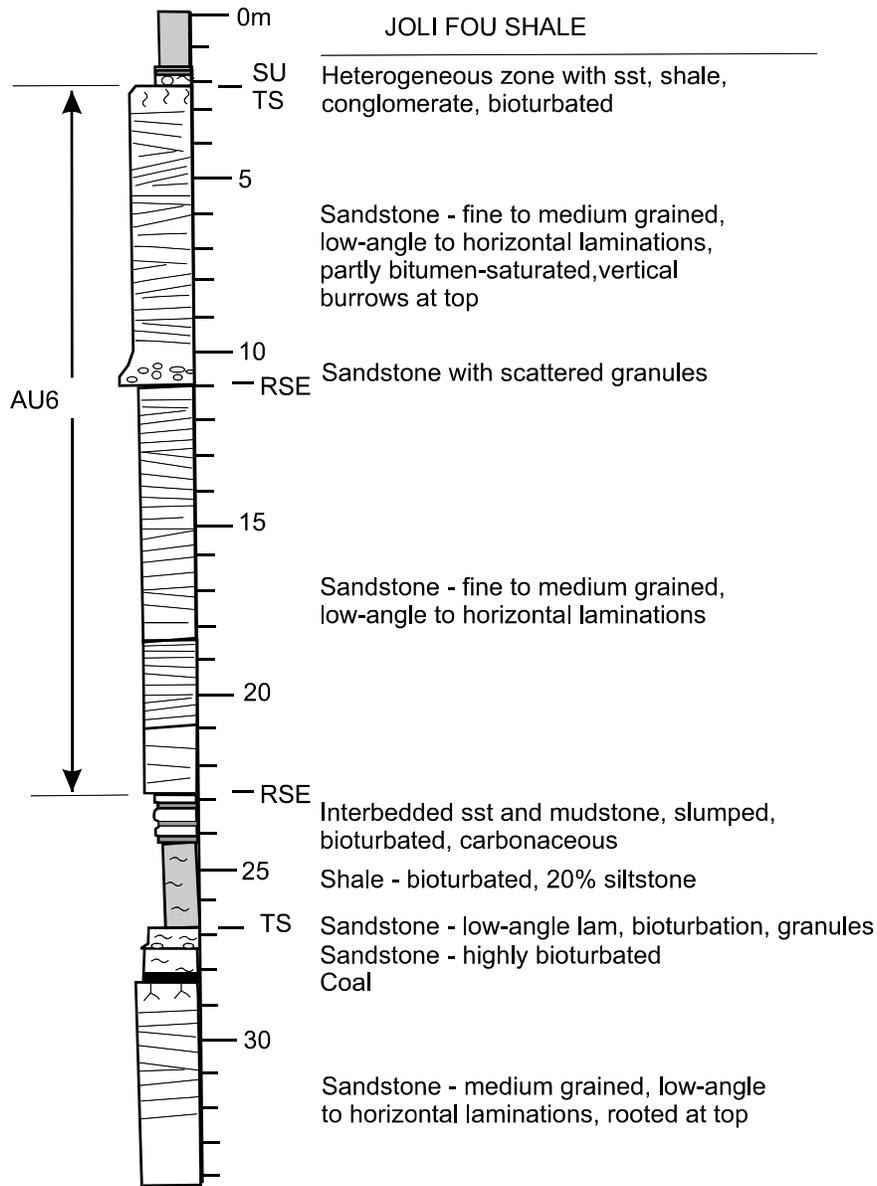
Figure 4: Core log showing amalgamated shoreface sands
