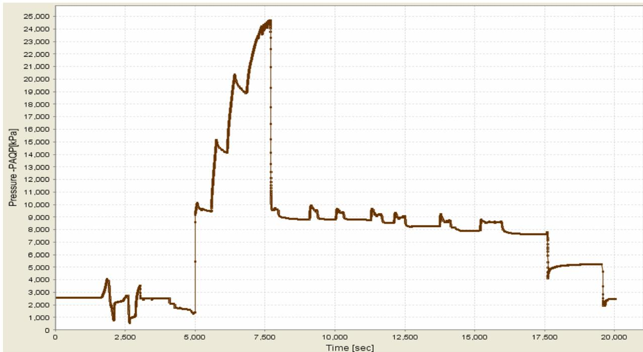
Figure3: Shale cap rock in situ stress test time/pressure results for SAGD cap rock in Western Canada.
