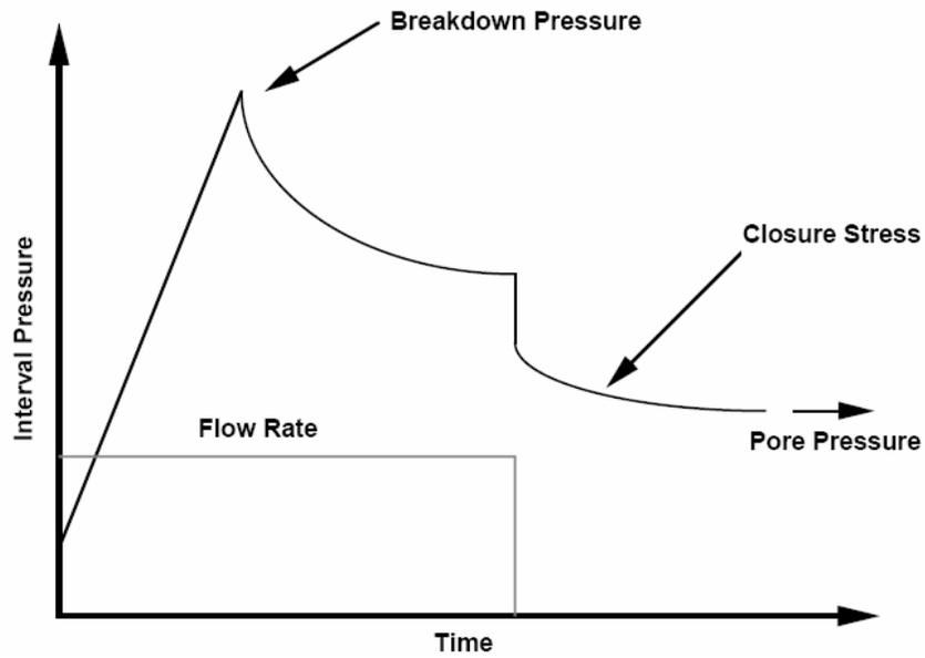
Figure2: Ideal time/pressure record for an situ stress test
