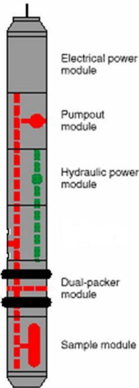
Figure1: Wireline stress testing tool configuration
