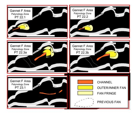
Fig. 4 Successive turbidite lobes filling a valley controlled by active salt tectonics
