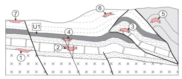
Figure 2: Schematic cross-section of the Cambrian-Ordovician St. Lawrence Platform and coeval Appalachian Humber Zone. The 7 conventional and one unconventional (U1) plays are presented. The plays 2, 3 and 4 are quantitatively assessed.
