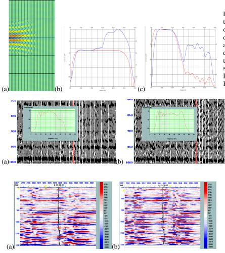
Figure 3. (a) Class 3 model gather shown in the time domain after applying ensemble operator in CDP domain (section was gained down to show the amplitudes unclipped). The amplitudes are severely distorted by applying ensemble operator in CDP domain. Note that the gradient has changed. (b) zero-offset trace spectrum and (c) far-offset trace spectrum. Red - without applying ensemble operator, Blue - after applying ensemble operator.
