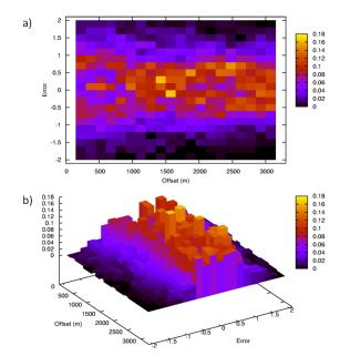
Figure 3: a) 2D view of the error PDFs for each offset. The distributions appear to become more Gaussian with increasing offset. b) 3D view of the error PDFs.
