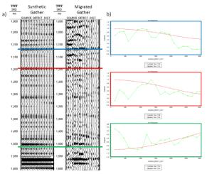
Figure 2: a) The synthetic (left) and migrated (right) CMP gathers. Note the random noise and multiples remaining in the migrated gather. b) Relative amplitudes for the synthetic and migrated gathers extracted along three time values.
