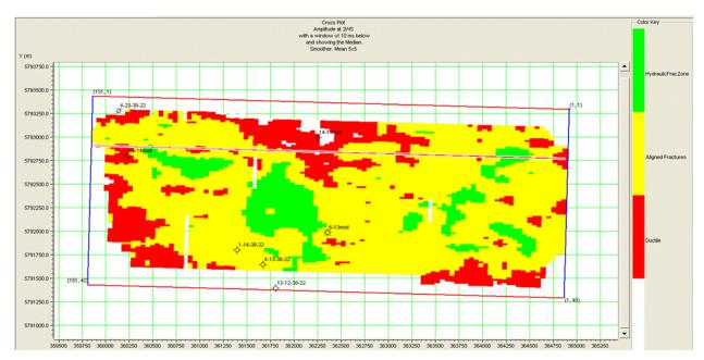
Figure 3: Map of 2nd White Speckled Shale showing zones highlighted in the crossplot in Figure 2. Green suggests where fracture swarms will form, red suggests the rocks are more ductile and thus less likely to fracture and yellow suggests where aligned fractures are likely to occur. Considerable variations are noted in the North-Central part of the survey, where the data suggests areas good and bad for hydraulic fracturing within about 100 m of each other.
