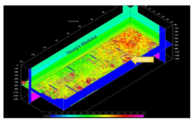
Figure 1: Colour background shows dynamic Young's Modulus estimated by our method, with its scale in MPa at the bottom of the Figure on this 10 km², 3D seismic volume. "Plates" (indicated by the arrow) show the Differential Horizontal Stress Ratio (DHSR). The size of the plate is proportional to the magnitude of the DHSR and the direction of the plate shows the direction of the local maximum horizontal stress. The long axis of the survey is E-W and survey area is 10 km².
