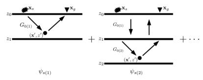
Figure 1: We give a schematic description of the first two terms in the series representation of the de-migration algorithm, where  $G_{0(l)}$  is the split-step Green's function for the  $l^{th}$  layer.
