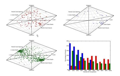
Figure 3. Source-type diagrams for three different hydraulic treatments from the same field. The histogram indicates the proportion of events with a given amount of double-couple component for the three datasets, the colour of the bars corresponds to the colour of the point in the source-type plots.
