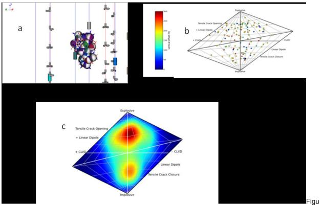
re 5. a) Distribution of events and their mechanisms associated with a reservoir based steaming injection program. Colour coding is as provided in Figure 1. b) Distribution of events on k-T source-type plot scaled by vertical position relative to the injection interval for steam injection related events. c) Contoured distribution of observed failure components for events related to a steaming operation.
