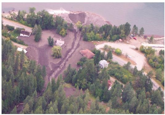
Figure 1. A debris flow initiated as a result of a localized heavy summer rain shower in a watershed following wildfire. Two homes were destroyed and the highway was closed for several days. (Source: D. Boyer, B.C. Ministry of Environment.)
