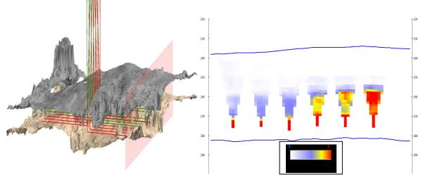
Figure 3: Left, proposed pads (producers in red, injector in green) between the median (P50) position of the top and base of the basal sands. Right, section going through the south pad (along the highlighted plane) after connectivity analysis.
