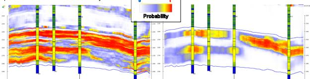
Figure 1: Bitumen probability (left) and thick continuous bitumen probability (right) in a random section (wells coloured by density, sands in yellow, shales in green and carbonates in blue)
