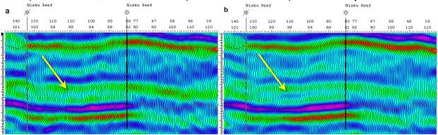
Figures 4: Reprocessing results (a) control reprocessing result, and (b) the full reprocessing as well as MWNI, and sparse Radon Transform with the aggressive mute. The Blueridge level is identified with a yellow arrow.
