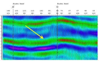
Figure 2: original (legacy) seismic line through a Nisku reef and Blueridge porosity. The amplitudes at the Blueridge level (yellow arrow) are much higher than expected from modeling.
