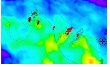
Figure 5. Microseismic monitoring data overlain with a Poisson's Ratio map from AVO inversion.
