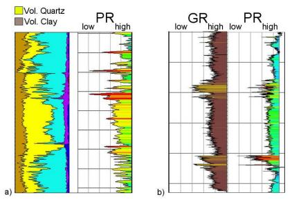
Figure 1: Log data that illustrate the correlation between low Vp/Vs ratio and/or Poisson's Ratio (PR) with increased sand-shale content, from a) a Western Canadian shale gas play, and b) a South Texas tight gas play where low gamma ray (GR) is taken as a proxy for increased quartz content.
