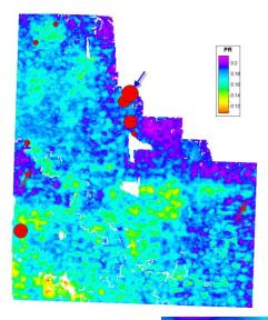
Figure 4. Map of median Poisson's Ratio value and porosity-height from 12 wells through the Lower Doig and Upper Montney. The red arrows highlight wells with very small porosity-height values and correspond in general to areas of higher Poisson's Ratio. The blue arrow highlights a well with a large porosity-height at the edge of the seismic data where the inversion is adversely affected by decreased fold.
