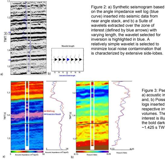
Figure 3: Pseudocolour a) acoustic impedance and, b) Poisson's ratio logs inserted into their respective inversion volumes. The zone of interest is illustrated by the bold dark horizon at ~1.425 s TWT.
