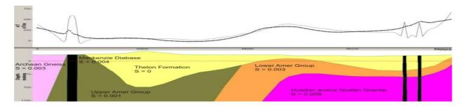
**Figure 4**: Extracted total magnetic intensity profile for EW-1. Top panel: Observed (heavy black dots) and computed (thin black line) magnetic anomaly. Bottom panel: computer generated geological model based on magnetic data. Different colours represent different susceptibility models for simplified major rock units as labelled here.
