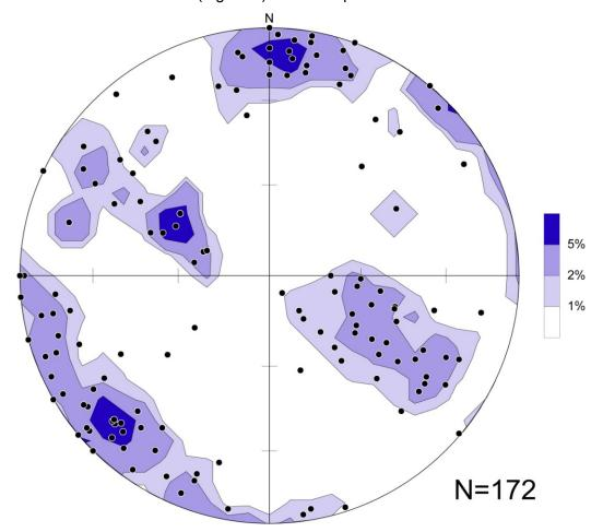
Figure 1: Stereoplot of poles to all surface fractures from scan lines in the South Peak area (western limb). Contours at 1%, 2% and 5% of data per 1% of net.
