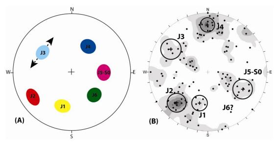
Figure 3: Comparison between the discontinuity sets detected using the COLTOP 3D software (A) and field survey (B) for the western fold limb (from Pedrazzini *et al.*, in press).
