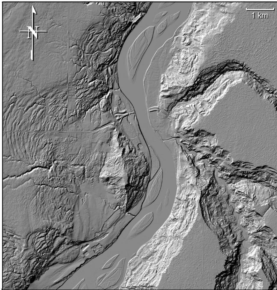
A sample of the bare-earth LiDAR digital elevation model that is used to map landslide features in the study area.
