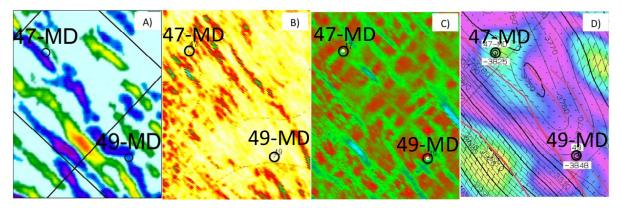
*Figure 3.* Top of reservoir amplitude maps calculated by A) Duplex Waves Volume B) Cube of Coherency, C) Most Positive Curvature by top of reservoir D) Map of Azimuthal Anisotropy. All methods define similar direction of anomalies, but DWM more accurately delineates the position and configuration of fractured zones than conventional methods.
