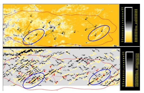
**Figure 1.** Comparison of an amplitude map of single-reflected waves from horizon Ia at the top of a reservoir (top) with that after duplex wave migration for the same horizon (bottom). The red contour shows the oil-bearing area. The most productive wells are outlined with blue ovals.
