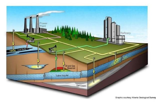
Figure 1: CO<sub>2</sub> capture from power plants and refineries and storage in saline aquifers, coal beds and salt caverns
