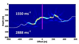
superimposed white line represents the true model contact. The P-wave velocities are for the soft sediments and the breccia unit respectively.
