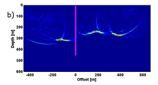
**Figure 4**: a) Preprocessed data from R-450 (muting and trace interpolation). Traces for small absolute offsets (<100m) were padded with zeros; **b)** Reconstructed sediment-breccia contact image from R450 using the migration method.
