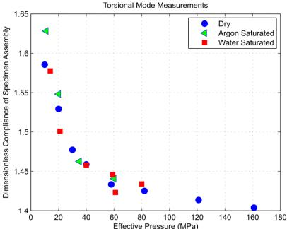
Figure 3. Dimensionless normalized compliance of the cracked Lucalox<sup>TM</sup> sample vs. effective pressure in torsion measured at 0.1 Hz.
