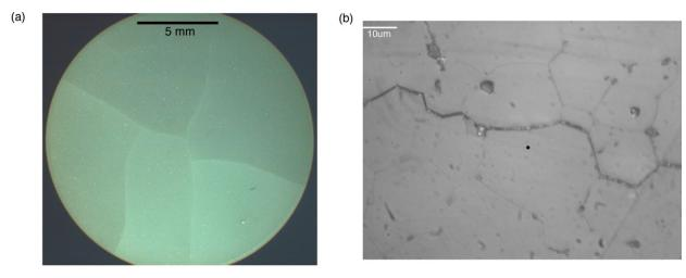
Figure 2. (a) Crack network in Lucalox polycrystalline alumina quenched from 1400°C into liquid nitrogen. (b) Representative micron-wide crack at higher magnification showing grain-boundary control of the thermal cracking.
