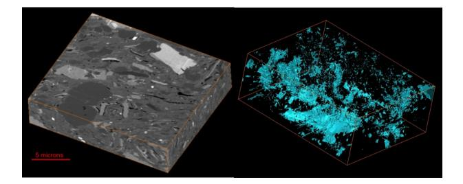
Figure 3: Left: FIB-SEM volume. Right: Pore Structure
