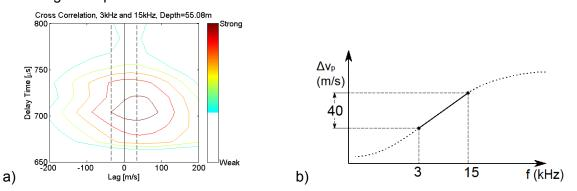
Figure 4: (a) Cross correlation of semblance plots in Figure 3a and 3b. Velocity lag of about 40m/s is observed. Weak correlations are shown in white. (b) P-wave velocity dispersion graph obtained from (a). Dotted line shows predicted trend by Pride (2005).
