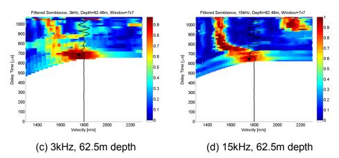
Figure 3: Semblance analysis. The plus sign "+" shows the manual velocity pick corresponding to the waveforms in Figure 2. Red and blue denote strong and weak coherency respectively. White regions contain coherency values of very weak signals. Black wiggle plot superimposed in each subfigure depicts the waveform recorded in channel 1.
