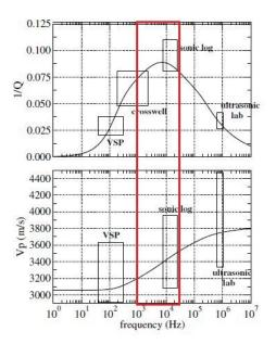
Figure 1: P-wave velocity dispersion model predicted (Pride, 2005). Red rectangular box indicates the frequency range, 1kHz – 30kHz, covered by this research project. Black rectangular boxes define the regions where measurements from Sams et al., 1997 are covered.
