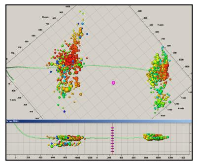
Figure 5: Relocated microseismic events from Stages 1 and 7 using the anisotropic model
