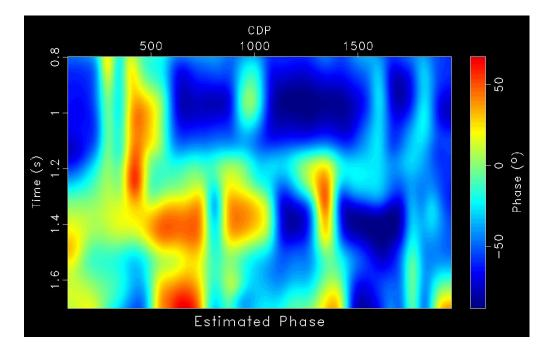
Figure 2: Estimated phase. Large variations in phase occur throughout the seismic section highlighting potential areas of interest. This happens for instance around CMP 450 between t=1.4 and 1.6 s but also below the pinch out at CMP 1300 at t=1.17s.
