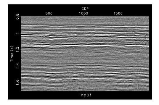
Figure 1: Stacked section displaying large variations in local frequency content. The coals are at *t*=1.05s. Variations in peak frequency can for instance be seen by comparing the section on the left and right of CMP 450 between 1.4 and 1.6 s. These variations result from frequency-dependent stratigraphic filtering through the overburden.
