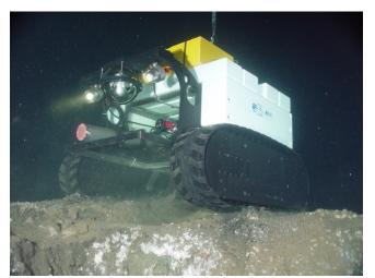
Figure 2: Crawler (Jacobs University, Germany) being deployed at Barkley Canyon gas hydrates
