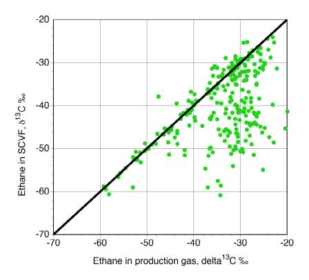
Figure 4. Comparison of ethane isotope values in production gas vs. SCVF gas.
