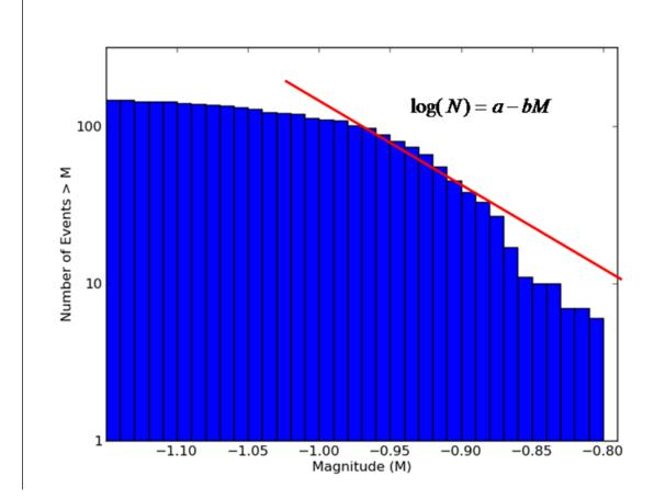
Figure 2. The frequency-magnitude distribution for the events in Figure 1. The b-value is calculated from the slope of the linear part of the FMD.
