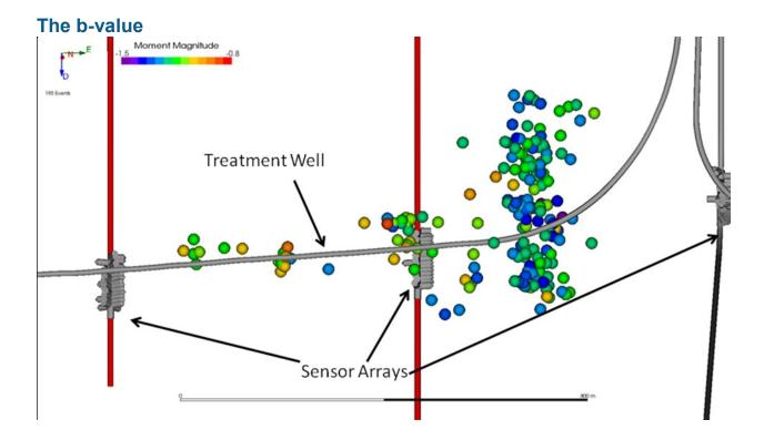
Figure 1. Distribution of events associated with stimulation in a horizontal treatment well (grey) utilizing a single array.
