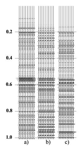
Figure 3: Stack results. a) 2m depth increment. b) 10m depth increment. c) 20m depth increment.
