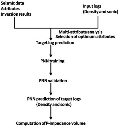
Figure 1: Workflow for neural network estimation of P-impedance
