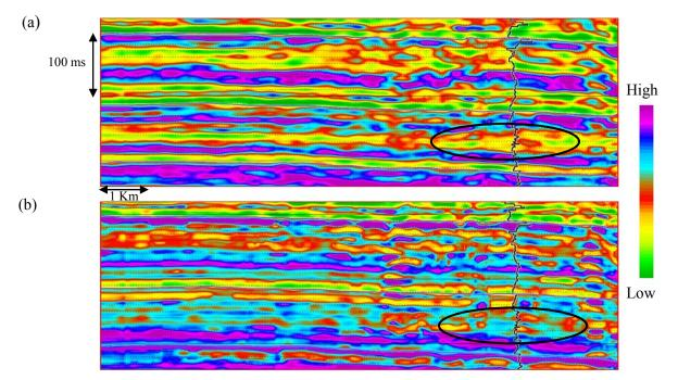
Figure 3: (a) P-impedance obtained from model-based post-stack inversion. (b) P-impedance obtained from PNN analysis. The P-impedance log is inserted. The black ellipse shows the zone of shale-sand play.
