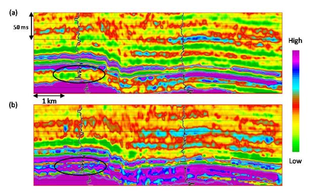
Figure 2: (a) P-impedance obtained from model-based post-stack inversion. (b) P-impedance obtained from PNN analysis. P-impedance logs at two locations are inserted. The black ellipse shown in the figure shows the zone of shale play. Notice the detailed and accurate correlation of the impedance values with the impedance log curves as seen on the neural network estimated impedance.
