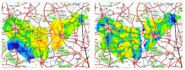
Figure 3. Resistivity-depth intervals derived from the full inversion of decoupled data. Depth Intervals 60-60 m, 120-140 m
