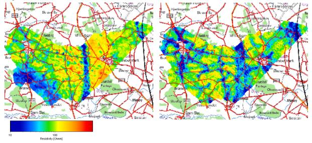
Figure 1: Inversion results obtained with completely unprocessed data., Depth intervals 60-80 m, and 120-140 m.
