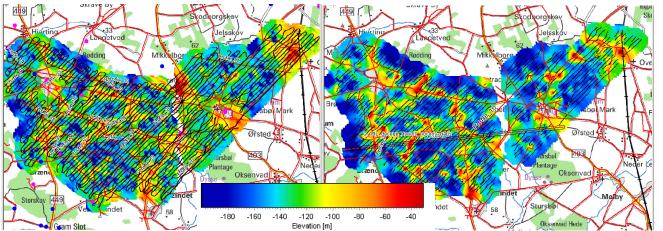
Figure 6. Elevation of the top of the good conductor (Paleogene clays), derived from decoupled data (left), and from data that was decoupled, averaged and denoised (right).
