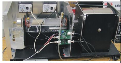
Figure 2: Theworking apparatus with faraday cage and signal processing boards.
