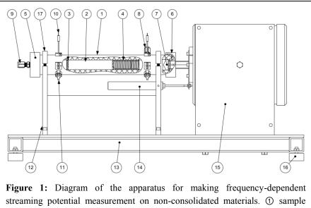
streaming potential measurement on non-consolidated materials. ① sample tube, ②sand sample, ③ polycarbonate disk, ④ spring, ⑤ output end-cap, ⑥ piston end-cap, ⑦ piston, ⑧ one-way valve (fluid in), ⑨ fluid out, ⑩ Ag/AgCl electrodes, ⑪ dynamic pressure transducers, ⑫⑬⑯⑰ rigid frame and vibration-damped feet, ⑭ LVDT, ⑮ dynamic shaker.
