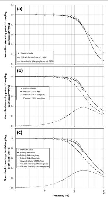
**Figure 3.** Normalized streaming potential coupling coefficient of Ottawa sand with 0.001 mol/L NaCl,  $T=24\pm0.8^{\circ}C$  as a function of frequency for (a) critically ( $\omega_t = 230 \text{ Hz}$ ) and variably (273 Hz) damped vibrational models (Thomson and Dahleh, 1998), (b) the model of Packard (1953), and (c) the model of Pride (1994) and the approximation of that model by Walker and Glover (2010).
