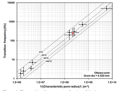
**Figure 4:** The transition frequency as a function of the inverse square effective pore size for Ottawa sand (red symbols) at  $T=24\pm0.8^{\circ}C$ . The dashed lines represent the theoretical result (Walker and Glover, 2010) at 4 different temperatures. The black symbols show all previously existing experimental data for capillary tubes, filters frits and rocks (Figure 6 of Walker and Glover (2010)).
