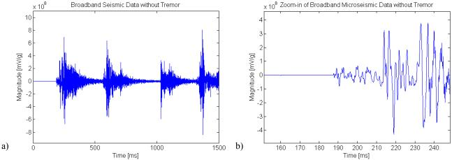
Figure 2: (a) Broadband seismic data without tremor. Multiple events are captured in this recording. The SNR is high, indicated by the quiet period at the beginning of the time series. The frequency content ranges from DC to around 2kHz. (b) Zoom-in view of (a). This is an example of classical P- and S-wave arrival with clear first-break.
