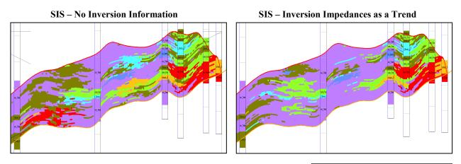
Figure 2: The left panel shows a SIS performed without the use of inversion information. In the right panel, the inversion impedances have been used as a trend. Note that the Lower Foreslope Facies (red) which are incorrectly placed in the left panel are correctly located when the inversion information is used.
