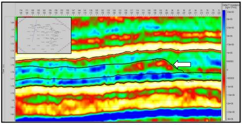
Figure 1: An arbitrary line from the inversion volume. The colors represent impedances as shown by the scale. The white arrow points to low impedances indicative of porosity development along the reef front.
