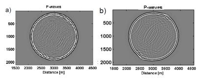
Figure 5. Snapshots of the propagating waves at 1s after source was triggered; a) uses the model with scale length of 100m (parallel to the dip direction), 10m (perpendicular to the dip direction).; b) uses the model with scale length of 6000m, 20m.
