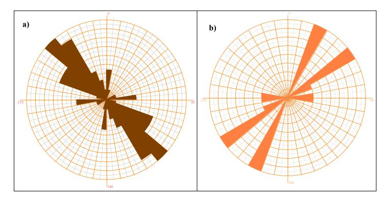
Figure 2: A rosette diagram showing a) the minimum horizontal stress direction (breakout) for all the 41 wells, the dominant stress direction is NW-SE b) the minimum horizontal stress direction for all the breakout intervals in wellbore 7-32-89-10W4; good example for variation in stress orientation with depth.
