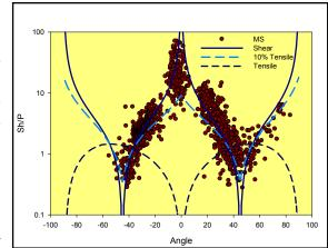
Figure 2. Composite amplitude ratio plot with various source mechanism models.
