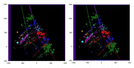
(source strength) density can be used Figure 5. Event density (left) and seismic moment density (right) (after
