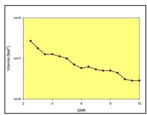
Figure 4. MS volume versus data confidence (SNR) (after Maxwell et al., 2010b).
