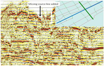
Figure 3: Structure stack of data after DSINTERP followed by 5D interpolation. Inset shows modified surface geometry map after inclusion of new shots along existing shot lines (via DSINTERP) together with inclusion of a previously missing segment of shot line (via 5D interpolation).
