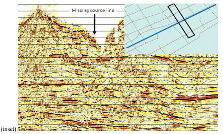
Figure 2: Structure stack of data after DSINTERP (main) together with modified surface geometry map showing inclusion of new shots along existing shot lines (inset).
