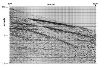
Figure 6. The application of AGC in the radial trace domain before linearly interpolating the trace gather leads to the greatest coherent noise attenuation, but at the cost of AVO relationships.
