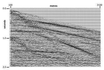
Figure 2. Application of radial trace filtering has attenuated most of the coherent noise on this gather, revealing many reflections.
