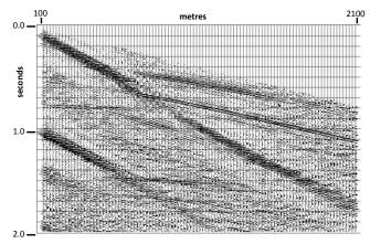
Figure 3. When receiver spacing is doubled during acquisition, coherent noise is aliased, making attenuation much less effective.
