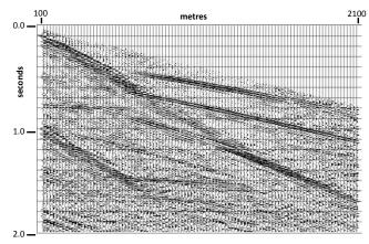
Figure 4. If LMO is applied to the trace gather to reduce coherent noise aliasing, attenuation is significantly more effective.
