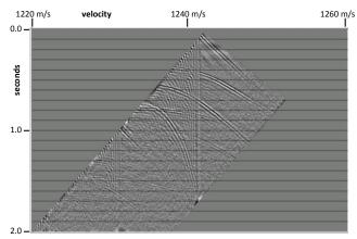
Figure A2. Radial trace dip transform of trace gather in Figure 1 after AGC. Noise amplitudes are dramatically reduced relative to reflections.
